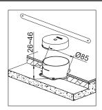
Make sure the distance between bottom of protector and top surface of tiles is within 26~46mm(top surface of tiles is between the MIN and MAX line on the protector). Drill Ø85 hole on the tile. Lay the floor tiles. Cut away the extending part of protector in accordance with the tile surface before install the faucet. The faucet's installation refer to the corresponding installation instructions.
