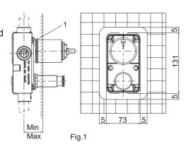
Connect Rc1/2" hot and cold supplies, showerhead and bath pipings to valve body as Fig.2 shown. Connect hot supply to the end on the left. For 880, do not connect the bath spout pipe. Supply enough tape or sealant.
