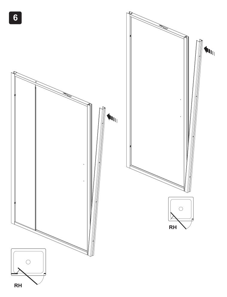
(a) Install the first wall channel over the door frame and hold in position.
