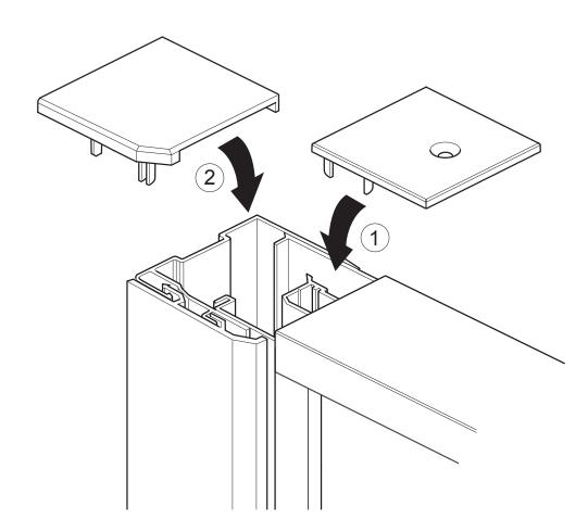
(a) Fit the plastic covers to the top of the extrusions. Modify caps if required.
