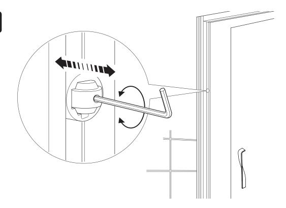
(a) If necessary, adjust the door catch as shown above.
