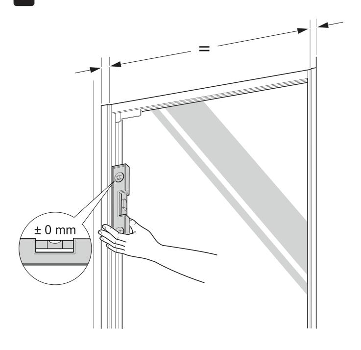
(a) Centralise the door frame within the wall channels, making sure that the door frame is square.
