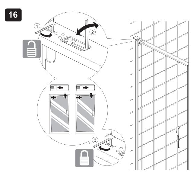
(a) If the door is out of square, adjust as shown above. If required, adjust the vertical seal until there is no gap for water to escape the enclosure.
