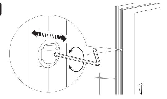
(a) If necessary, adjust the door catch as shown above.
