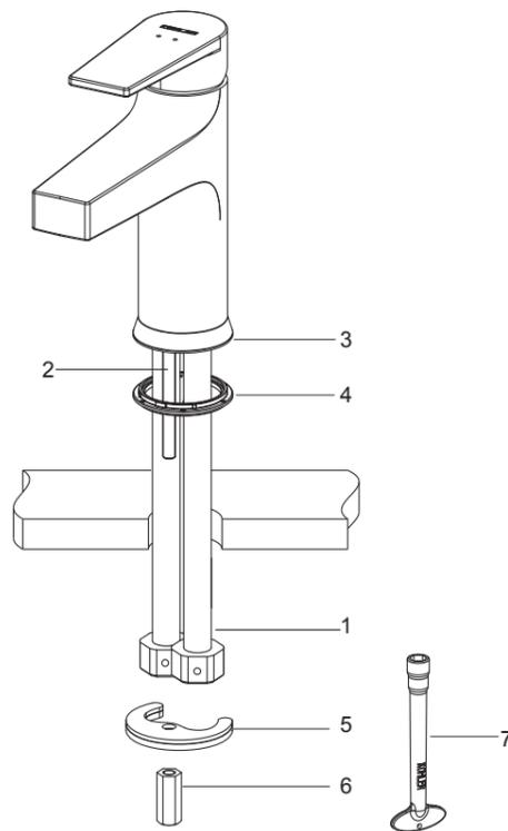
Install the mounting stud(2) onto the faucet body base(3).
