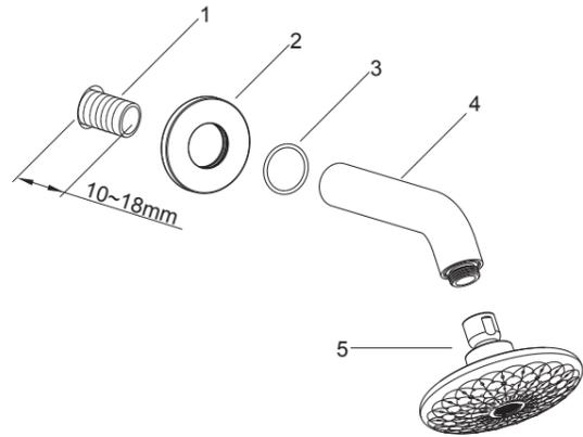
Be sure the O-ring(3) is in the escutcheon(2), apply a ring of plumbers putty around the back surface of the escutcheon. Apply tape or thread sealant to the nipple threads, install the escutcheon and the shower arm(4). Adjust the shower arm downwards, tighten with a strap wrench. Adjust the escutcheon and make sure it against the wall. Remove any excess putty.
