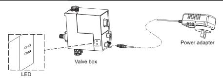
Connect the power adapter to the valve box as shown, and then connect the power adapter to the power socket. When the LED on the valve box is green, which indicates that the power supply is connected.
