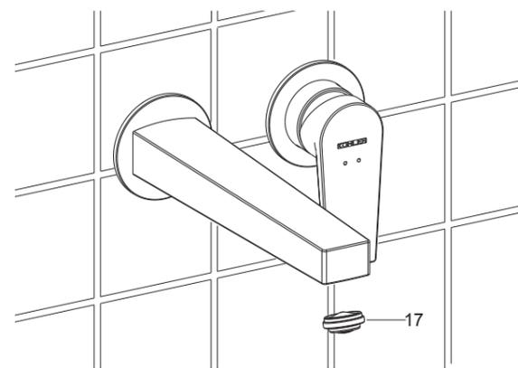
Ensure that all coupling nuts are tight. Ensure that the lever handle is in the off position.
