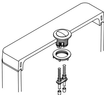
4 Fit the lid and test the buttons. Adjust the rods as required.
