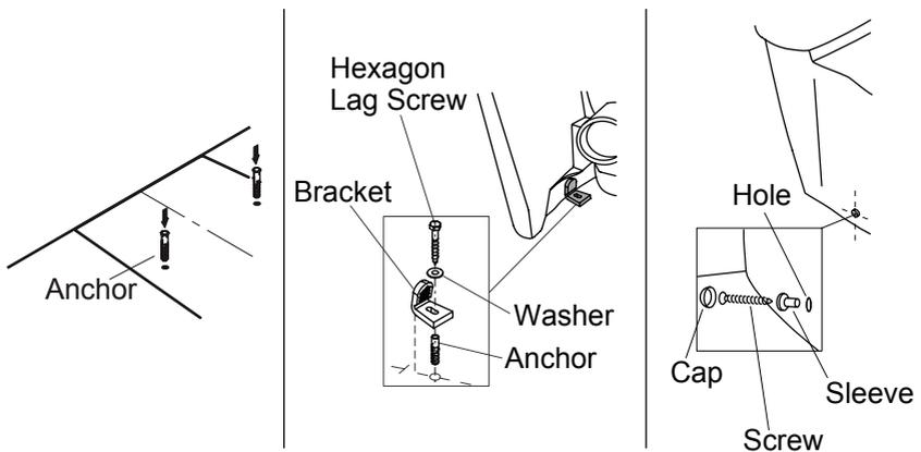
5 Place a washer onto each of the hexagon screws and fix the brackets to the floor.
