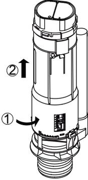
2 Assemble flush valve by pushing straight down into the canister and turning clockwise.
