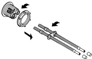
2 Using the push rod, measure the distance between the flush valve and the top of the cistern lid. Mark this length and cut the push rod to length.
