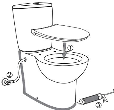
2 Make final connection of water supply hose to shut-off valve. Test the system for leaks.
