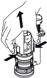
2 Assemble flush valve by pressing it into the flush valve so it snaps into place.
