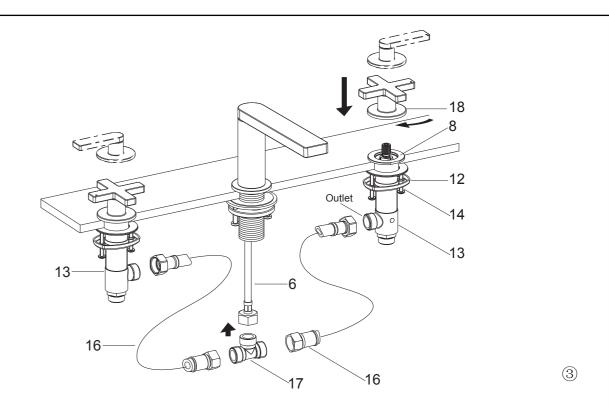
Adjust the outlets of side bodies to connect hoses easily. Secure the side bodies by tightening screws(14) with screwdriver.
