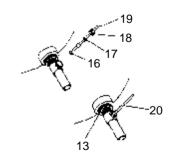
**NOTE:** Do not reposition the drain after the locknut is tightened, or you may break the putty seal.
